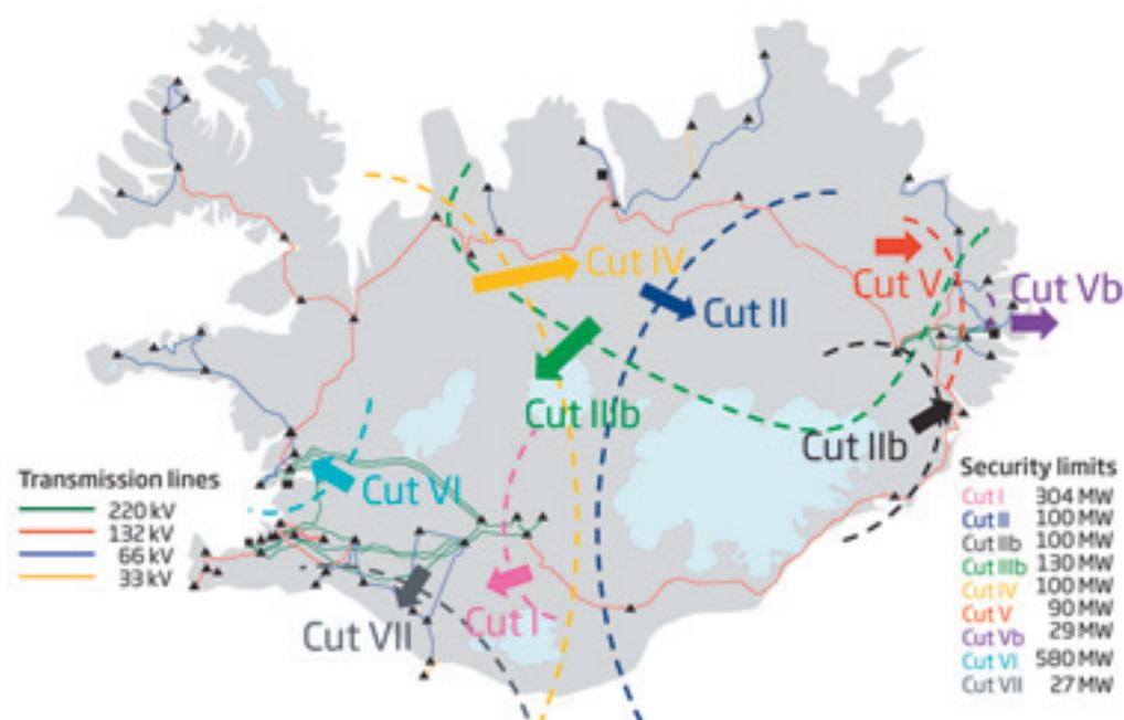
We constantly monitor transmissions through nine defined transmission cut-planes in the grid, shown on the above map. When grid disturbances occur, the risk of an outage is heightened when the level of transmission through a cut-plane nears or exceeds security limits. The graph below shows the level of transmission through eight cut-planes for the whole of 2015. As can be seen, the grid's
